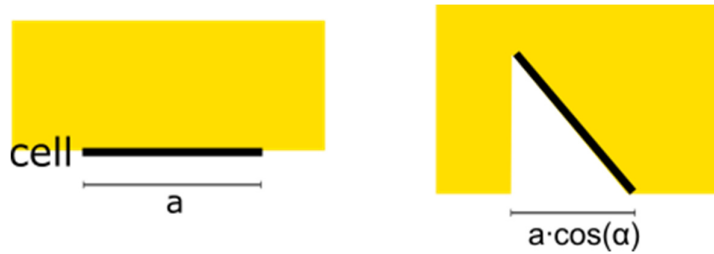
Figure 3: Schematic illustration of the illumination cases under various incident angles used during the current-voltage (JV) measurements. An overall spot size of 10 cm x 10 cm is illuminated, which is two orders of magnitude the size of the illuminated solar cell area under normal incidence conditions. A variation of the angle leads to a reduced photon flux per unit area (reduced “effective illuminated device area”) following the “cosine law” A(\alpha)=A_0 \cdot \cos(\alpha) . [31,32]
